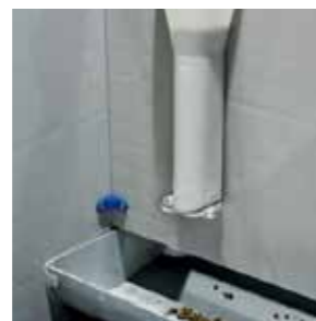
Straw-pellet dispenser above wet-feed trough.
