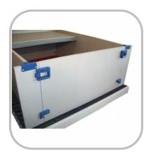
Perhaps a broad gate, which can be opened in both ends and operated with one hand is preferable? Ikadan has developed a Multi-gate-latch functioning as handle, hinge and lock. – By lifting the latch the handle becomes free of the lock and the gate is lifted out of the hinge fitting.
